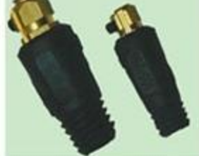
Terminal Plug TSKM 25 (10-25mm², 200A) Terminal Plug TSK 70 (35-70mm², 400A)
